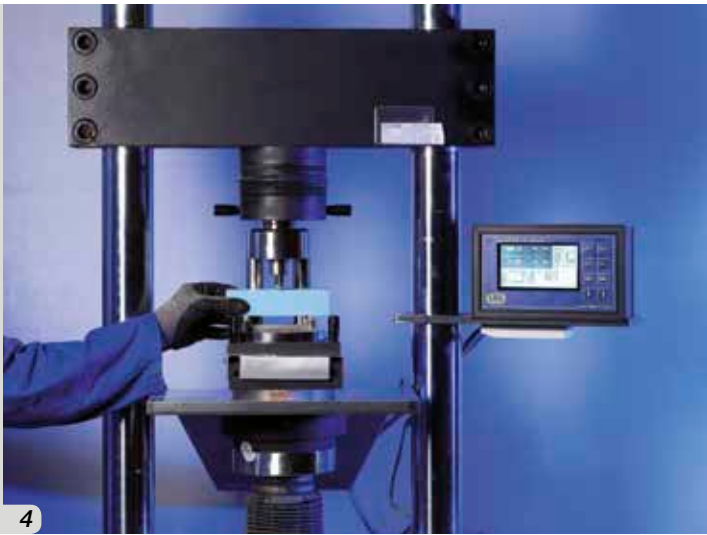
Fig. 4 - Test to measure the flexural strength of a sample of cementitious grout Fig. 5 - Water absorption test
