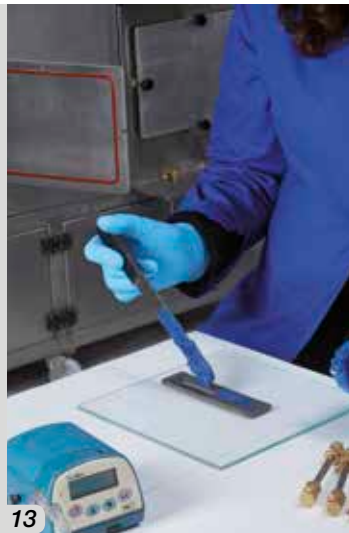
Fig. 12 - Environmental simulation chambers available at the Mapei R&D laboratory Figs. 13_14 - Test to measure VOC emissions
