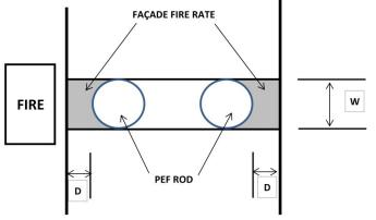
Ratio of joint depth (D) to the width (W) 5mm to 10mm joint ratio is -1:1 Depth (D) of joint over 10mm is - width (W) divided by 3 plus 6mm
